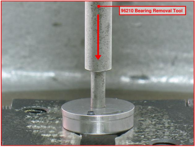
**6.** Use the **96210** Bearing Removal Tool and the arbor press to remove the **02696** Bearing from the rear bearing plate.
