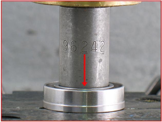
**6.** Use the **RAISED OUTSIDE DIAMETER** of the **96242** Bearing Press Tool and the **94232** Arbor Press (#2) to install the **02696** Bearing into the **02673** Rear Bearing Plate.
