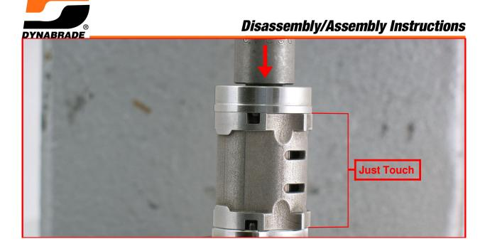
**8.** Use the **RAISED INSIDE DIAMETER** of the **96242** Bearing Press Tool and the arbor press to install the rear bearing and plate onto the rotor. **Notice:** Carefully press the bearing and plate down until it <u>just touches the cylinder</u>. This will establish a close fit between the bearing plates and the cylinder.
