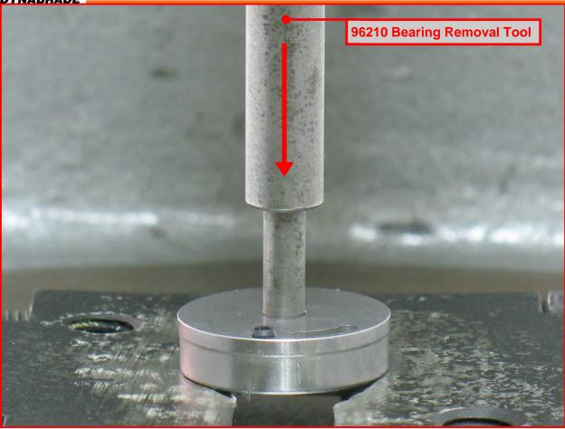
**6.** Use the **96210** Bearing Removal Tool and the arbor press to remove the **02696** Bearing from the rear bearing plate.
