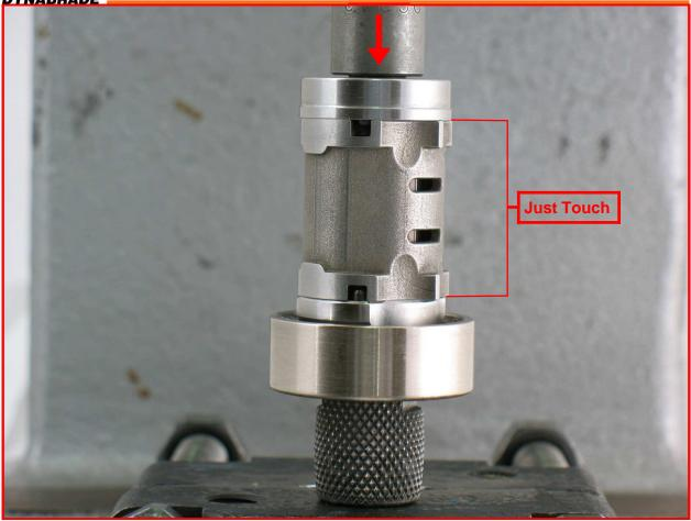
8. Use the **RAISED INSIDE DIAMETER** of the **96242** Bearing Press Tool and the arbor press to install the rear bearing and plate onto the rotor. **Notice:** Carefully press the bearing and plate down until it <u>just touches the cylinder</u>. This will establish a close fit between the bearing plates and the cylinder.
