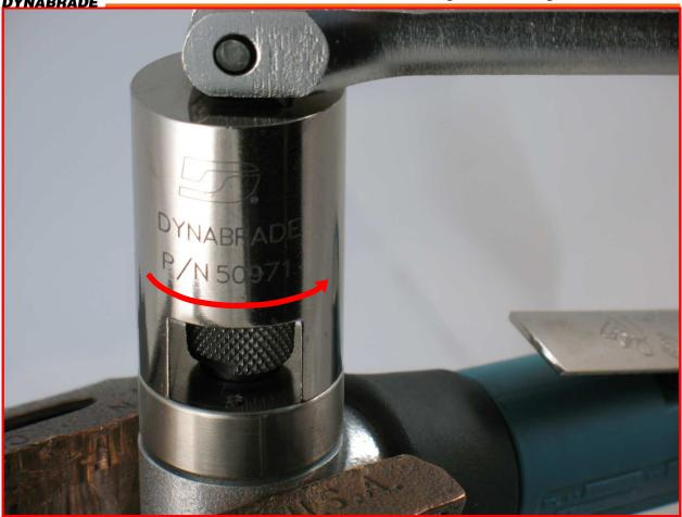
**3.** Use the **50971** Lock Ring Tool or an adjustable 3 mm pin spanner wrench to remove the **15106** Exhaust Cover. Turn counterclockwise.
