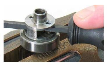
9. Use the arbor press, and a 5/16" flat-end drive punch as a press tool to push the planetary
