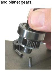
6. Use a 5/16" flat-end drive punch as a press tool to push the planetary carrier out of the 54520 Bearing.
