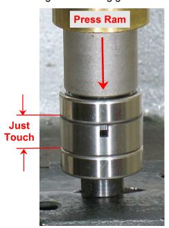
Install the planetary reduction into the adapter and/or planetary housing or gear case.
