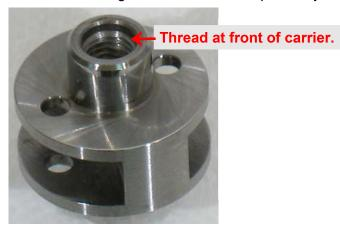
**2.** Apply a small amount of Loctite #271 (or equivalent) to the adapter or pinion thread.
