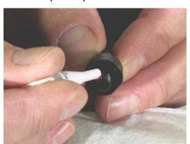
**3.** Apply the **95542** Grease (or equivalent) to the needle bearings in the planet gears.
