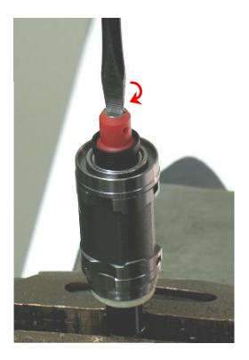
7. Use a 3/32" (2.38 mm) diameter flat-end drive punch as a press tool to push the rotor out of the **02696** Bearing.
