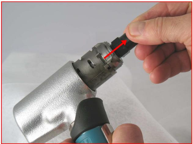
Pull the motor out of the housing.
