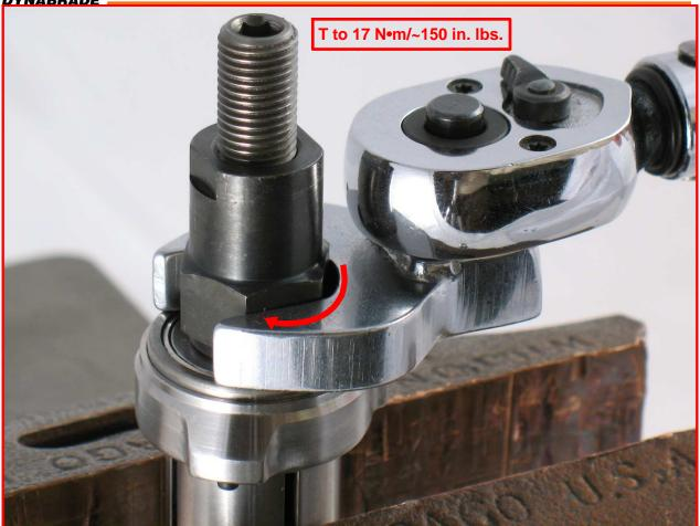
3. Use a 17 mm socket or crowfoot, and a torque wrench to tighten the **04081** Rotor Nut. (**T** to 17 N•m/~150 in. lbs.)
