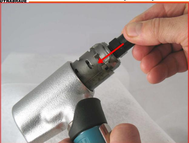
8. Install the motor assembly.
