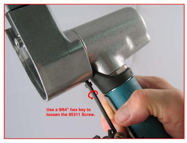
1. Use a 9/64" hex key to loosen the 95311 Screw. Remove the motor from the belt housing.
