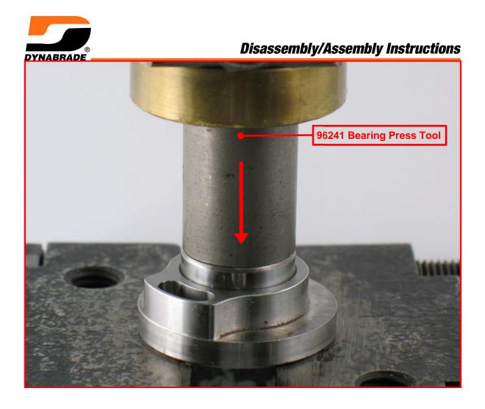
**5.** Use the **RAISED OUTSIDE DIAMETER** of the **96241** Bearing Press Tool and the arbor press to install the **01015** Bearing. **Notice:** Press the bearing all the way into the plate.
