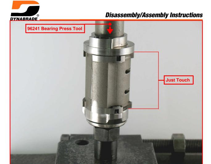
**7.** Use the **RAISED INSIDE DIAMETER** of the **96241** Bearing Press Tool and the arbor press to install the bearing and plate.
