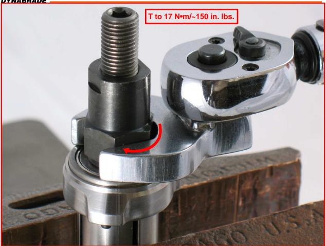
3. Use a 19 mm crowfoot and a torque wrench to tighten the **01708** Rotor Nut. (**T** to 17 N•m/~150 in. lbs.)
