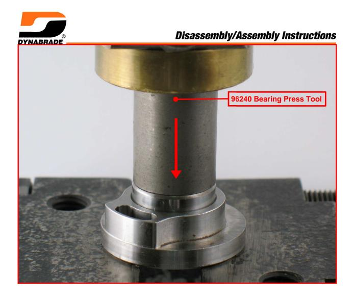
**5.** Use the **RAISED OUTSIDE DIAMETER** of the **96240** Bearing Press Tool and the arbor press to install the **02649** Bearing. **Notice:** Press the bearing all the way into the plate.
