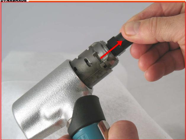
Pull the motor out of the housing.
