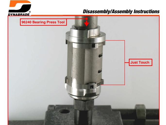
**7.** Use the **RAISED INSIDE DIAMETER** of the **96240** Bearing Press Tool and the arbor press to install the bearing and plate.
