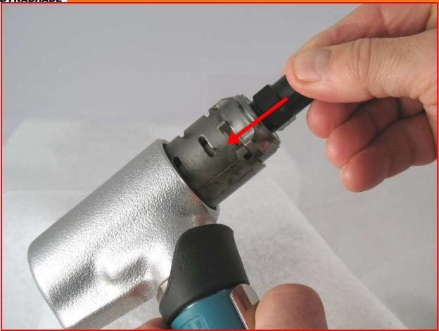
8. Install the motor assembly.
