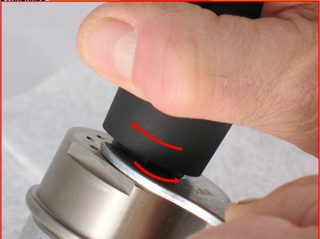
**10.** Use a 19 mm wrench to hold the motor spindle. By hand, or with groove pliers, grasp the drive wheel and install it. Turn clockwise.
