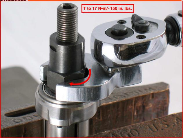
Use a 19 mm crowfoot and a torque wrench to tighten the 01708 Rotor Nut. (T to 17 N•m/~150 in. lbs.)
