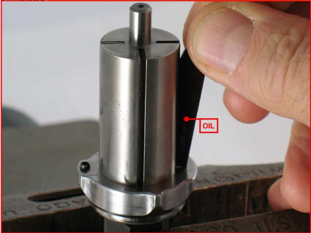
4. Apply the **95842** Dynabrade Air Lube 10W/NR or equivalent to the **01185** Vanes and install them into the rotor.
